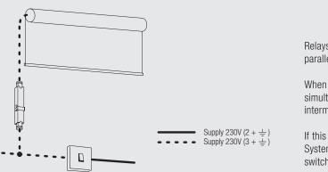
Relays (5736) must be used if **multiple systems** are connected in parallel.
