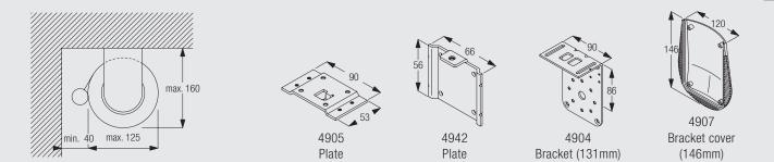
The fitting key parts shown above are part of bracket set 4949.
