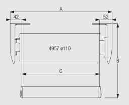
A: system width B: system drop C: fabric width
