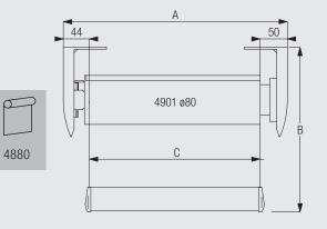
A: system width B: system drop C: fabric width
