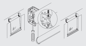
Vertical adjustment of the system (A) allows the headtube to be levelled.
