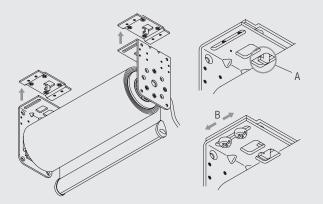
The brackets can be laterally adjusted by up to 18mm.
