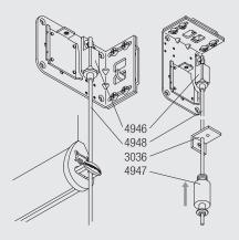
4946 Top fastener 4948 Wire rope (1.5mm) 3036 Bracket 4947 Bottom fastener
