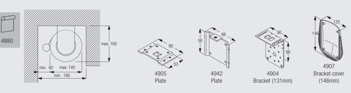
The fitting key parts shown above are part of bracket set 4949.
